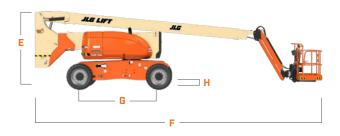
Platform Width 36-in / 0.91-m Platform Length B. 96-in / 2.44-m Machine Width 8-ft 2-in / 2.48-m Tailswing D. 2-ft 6-in / 76-cm Machine Height 9-ft 10-in / 3.0-m E. Machine Length 36-ft 6-in / 11.13-m F. Wheelbase 10-ft / 3.05-m H. **Ground Clearance** 11-in / 28-cm
