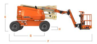
Platform Width 30-in / 0.76-m Platform Length 72-in / 1.83-m В. C. Machine Width 7-ft 8.6-in / 2.35-m Tailswing D. Zero E. Machine Height 7-ft 5.3-in / 2.27-m Machine Length 21-ft 6.9-in / 6.57-m G. Wheelbase 7-ft 9-in / 2.36-m **Ground Clearance** 16.4-in / 41.7-cm
