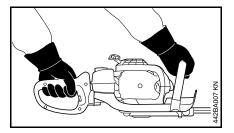
Left hand on the control handle and right hand on the front handle.
