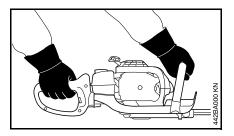
Right hand on the control handle and left hand on the front handle.
