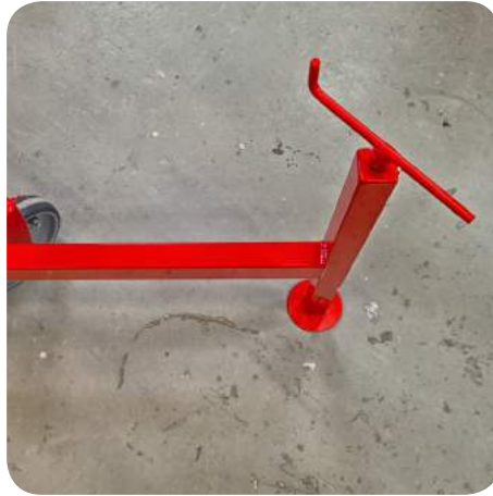
STABILISERS ENABLING OUTDOOR RATING EN 280/2013 12.5 M/S WIND
