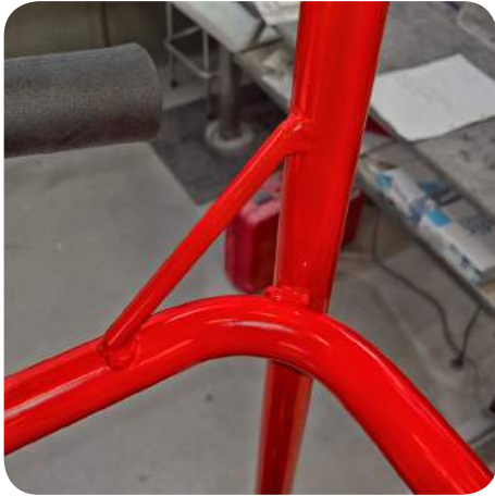
SAFETY HARNESS CONNECTOR POINTS EN 280/2013 3kN FORCE
